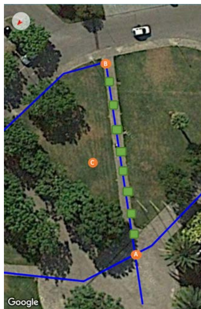
Figure 6. Example of filling intermediary points to determine the closest segment to a given point
