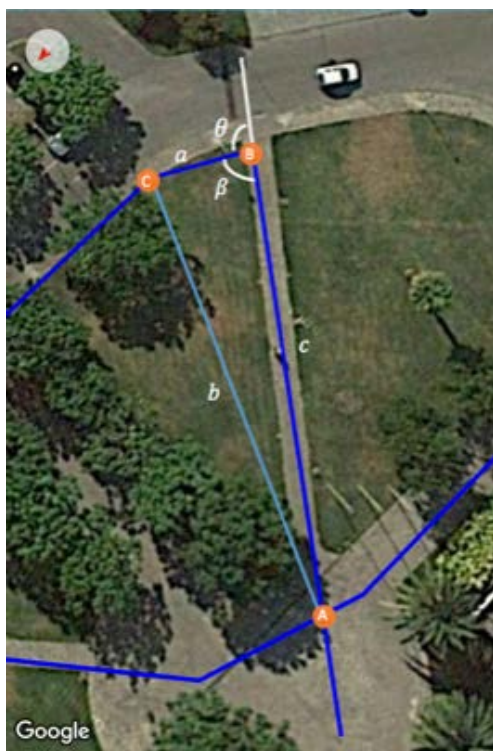
Figure 7. Angle calculation between two line segments
