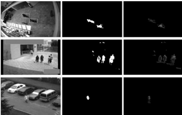
Figure 8. Comparison of Character Intrusion Detection Effects
