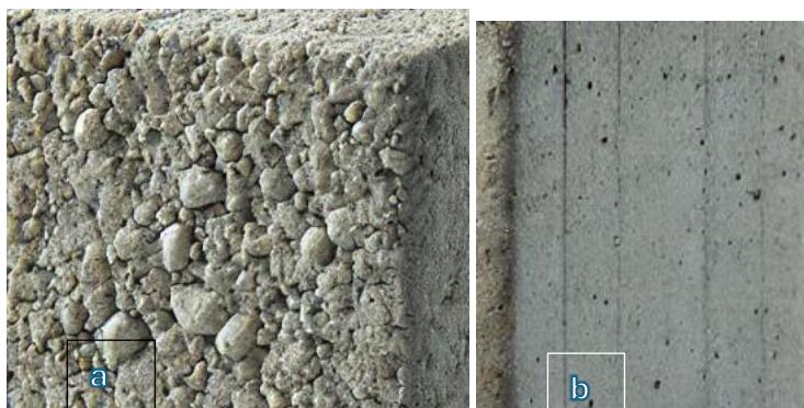
Figure 1 a.Foam Concrete (600 kg/m 3 ) b. Foam Concrete (1200 kg/m 3 )
