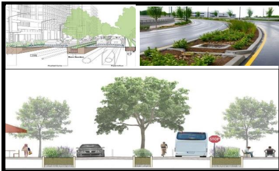
Figure (9): The central median and its treatments for green infrastructure for rainwater and irrigation
