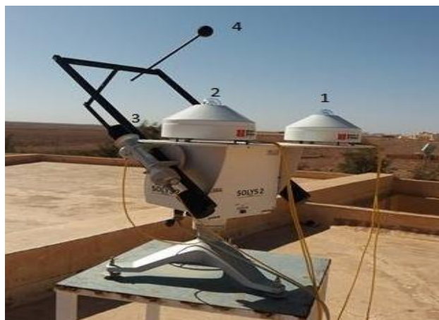
Figure 5. Instrumentation station for measuring the global, the direct and the diffuse solar radiation: (1) Pyranometre for measuring the diffuse. (2) irradiance Pyranometre for measuring the global solar irradiance. (3) Peryheliometer for measuring the directirradiance component. (4) The ball used to permanently hide the Pyranometer.
