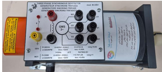
Figure 3 The synchronous motor
