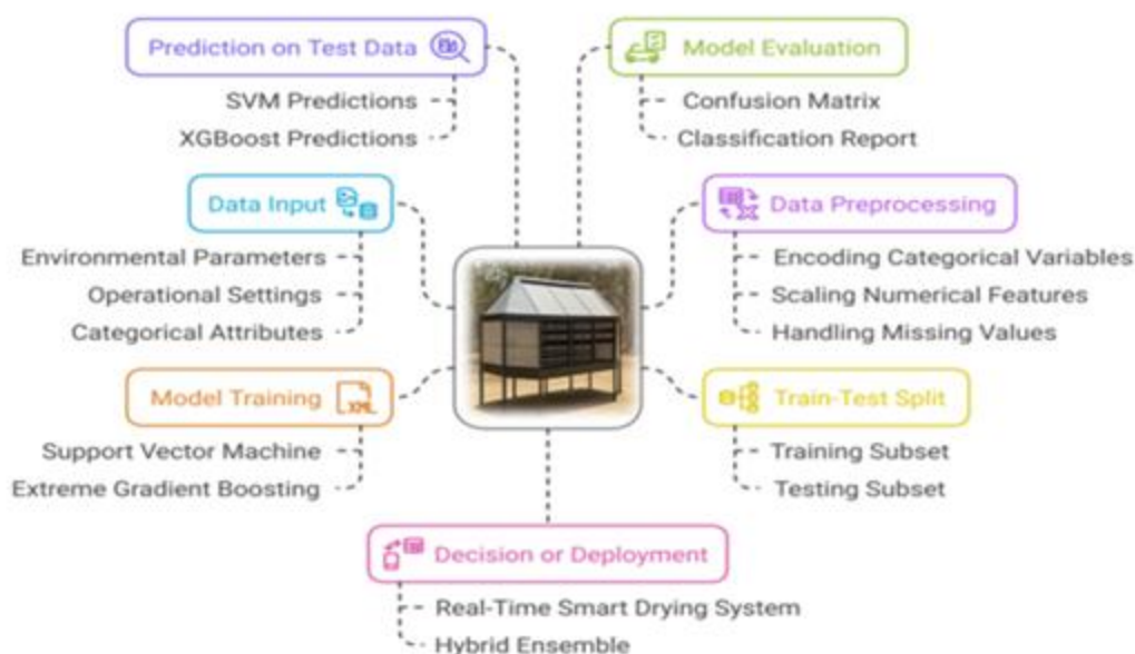
Figure 2. Flowchart of the Drying Status Classification Using SVM and XGBoost.
