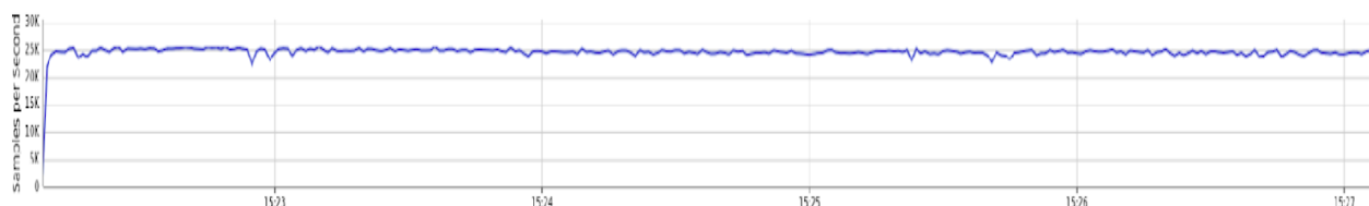
Figure 15: Single UDP DDoS attack impact on sFlow-test as Samples per second
