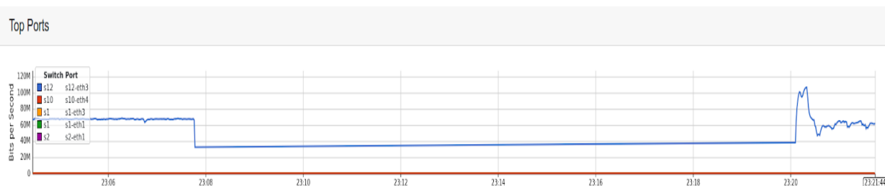
Figure 12: Top switch flows (anomalous traffic due to UDP DDoS attack in M bps)
