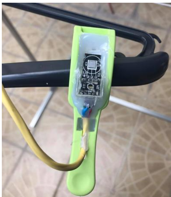
Figure 7. Humidity sensor attached at the clothespins
