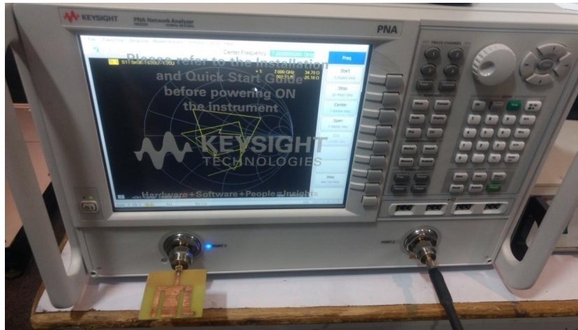
Figure 9: Measured input impedance of the proposed antenna with notch at 7 GHz
