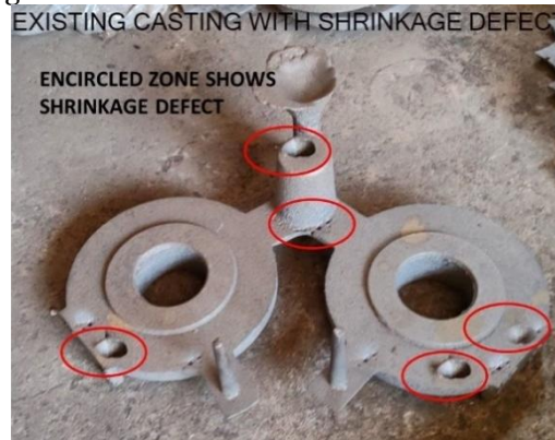
Figure 1 Shrinkage defect in casting
