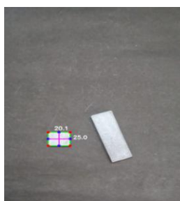
Figure 3.1 Image for measurement of length and width of sample D kept aligned with sample A as reference block. The output value is as given by developed algorithm.
