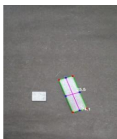
Figure 3.1 Image for measurement of length and width of sample D kept aligned with sample A as reference block. The output value is as given by developed algorithm.
