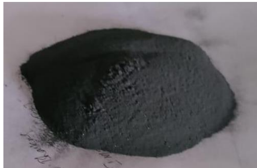
Fig.2 Silicon Nitride ( \text{Si}_3\text{N}_4 )
