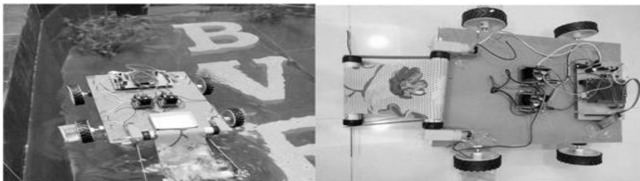
Figure 3 Prototype of AI-based river cleaning robot
