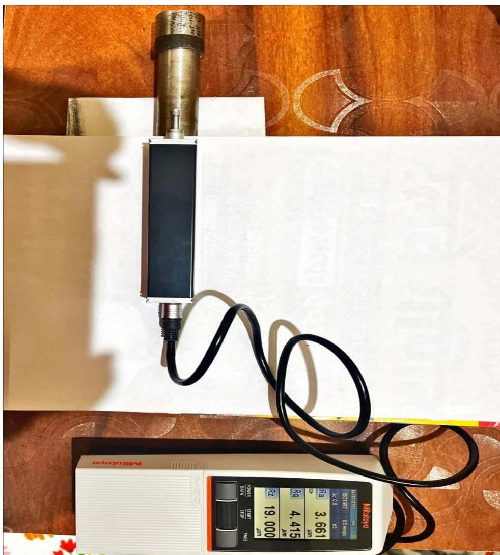
Fig. 2. Schematic of the experimental setup for measurement of surface roughness parameters.
