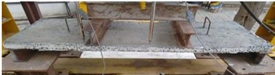
LVDT at Center and support
