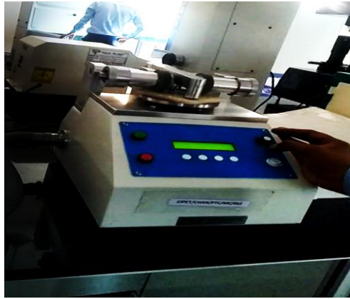
Figure 2. Pin-on-disc tribometer for Wear Testing.
