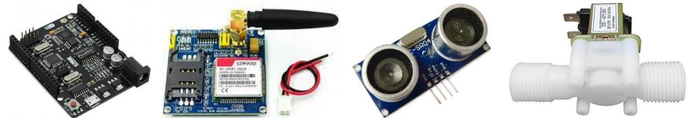
Figure 2: The ARDUINO WIFI ESP8266 board, GSM SIM900A module, Ultrasonic distance sensor and Solenoid valve
