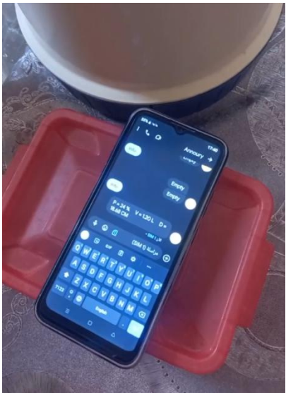
Figure 7: SMS received by the user for (LED red ON, P = 24%, "Empty")
