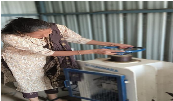
Figure 3 - Compressive strength testing on CTM
