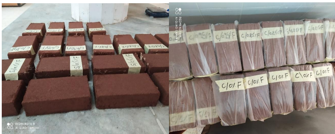
Figure3. Some of the SEB specimens, with different stabilizers (cement, Ground flaxseed and lime) and fibers contents.
