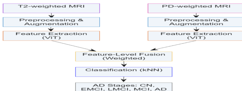
Figure 1 Block diagram of the proposed feature-level fusion approach based on Vision Transformer (ViT).
