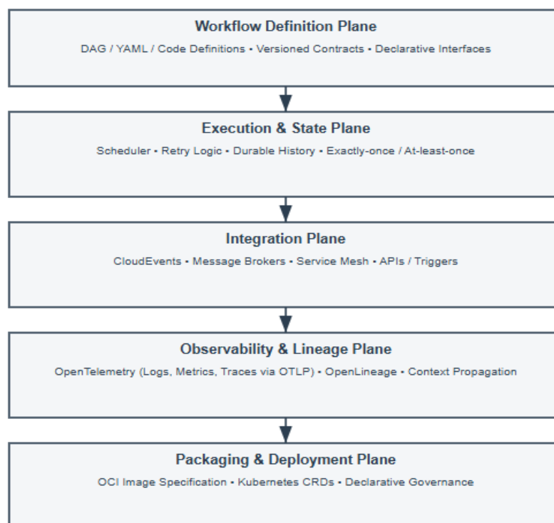
Figure 2: Five-Plane Interoperability Architecture for Vendor-Neutral Workflow Orchestration
