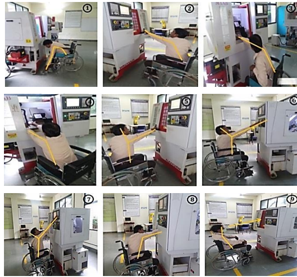
Fig 2.3: Ergonomic Risk Postures for Seated CNC Operators: 1. Lifting Work piece from Ground, 2. Opening Safety Door, 3. Loading Work piece, 4. Loading Tool, 5. Closing Safety Door, 6. Operating Key Panel, 7. Operating Control Panel, 8. Adjusting Tool, 9. Monitoring Control Panel
