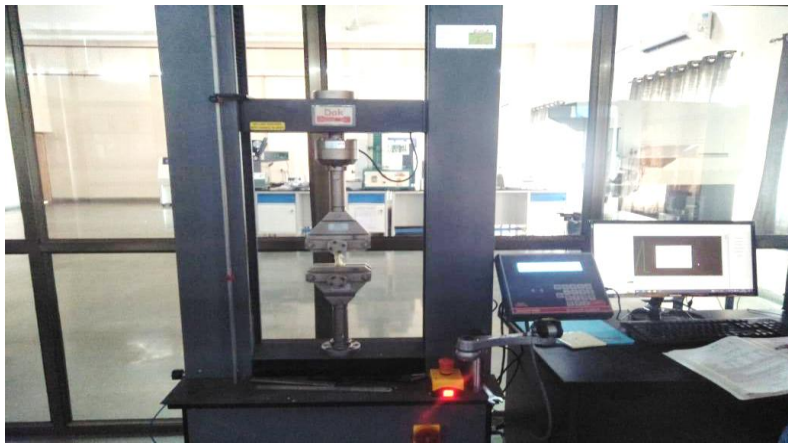
Figure 3. UTM Machine to check the Tensile Strength of Samples.
