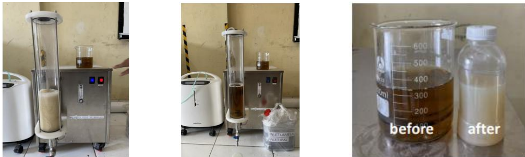
Figure 4. Comparison of wastewater before and after PFB implementation
