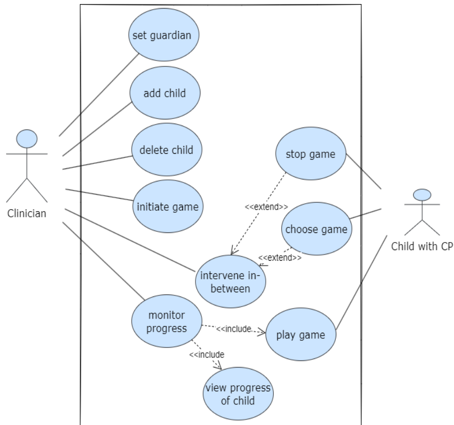
Fig. 2: Use case diagram for VR based rehabilitation
