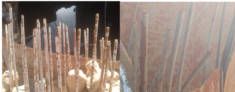
Fig. (3): Shows pre-stressed wire ductile fracture for burst pipe
