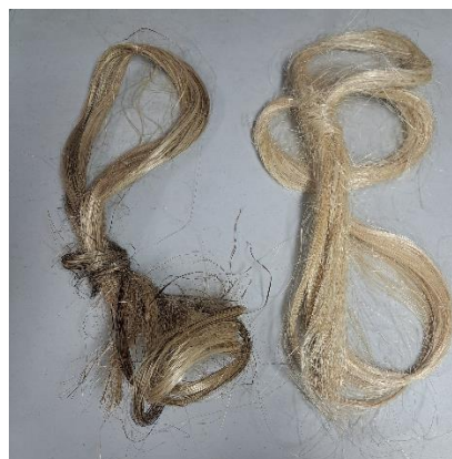
Figure 2. Grades S2 (left) and S3 (right) Abaca Fibers
