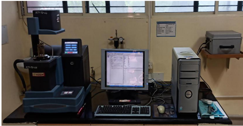
Fig. 2: Experimental setup of DMA.
