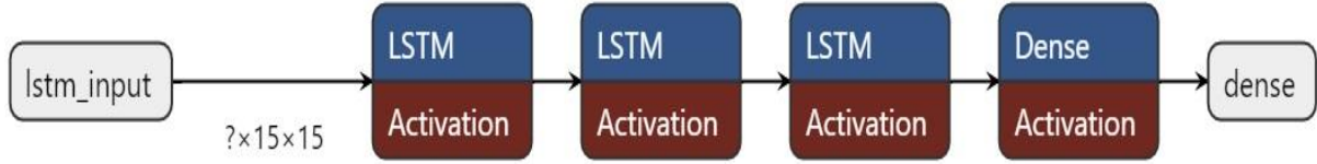
Fig.7 LSTM model architecture used for KWS
