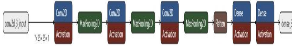
Fig.6 CNN model architecture used for KWS
