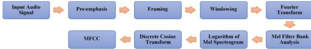
Fig. 4 . MFCC feature extraction process
