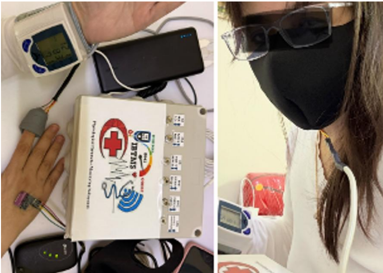
Figure 19: Physiological signs measurement using the IBTMS prototype
