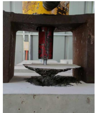
Figure 3 (c) Pull-out Strength Test
