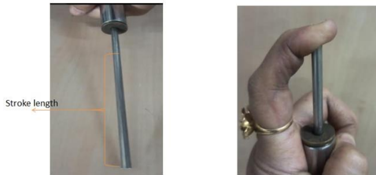
Photograph 2: Extended and retracted position of LVDT
