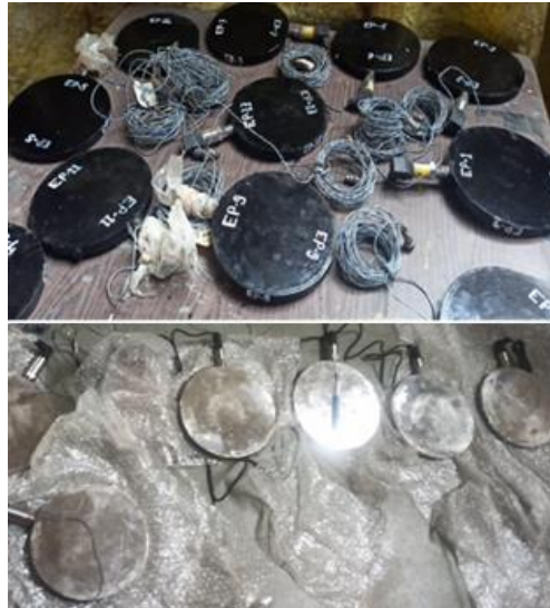
Photograph 3: View of the old black EPC recovered from the previous study road model and new silver EPC
