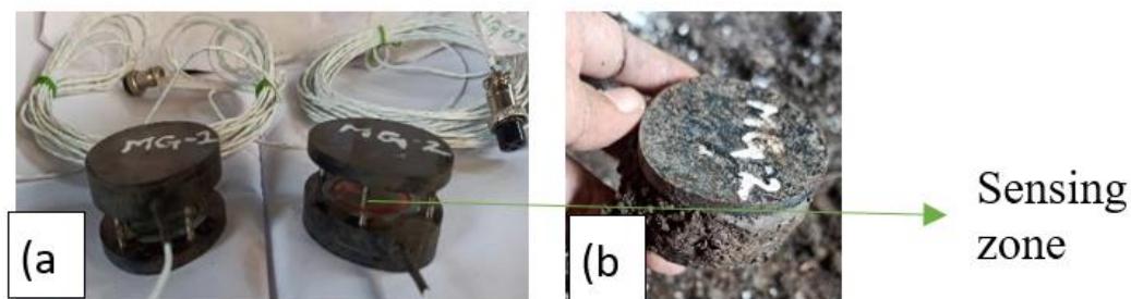
Photograph 5: (a) Moisture gauges and (b) Sample filled in moisture gauge
