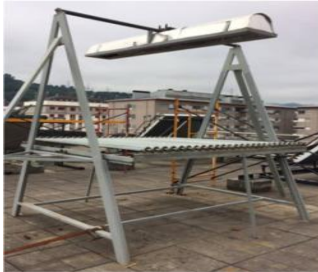
Figure 12 Experimental setup of a small-scale LFC with an open-loop solar tracking system [74].
