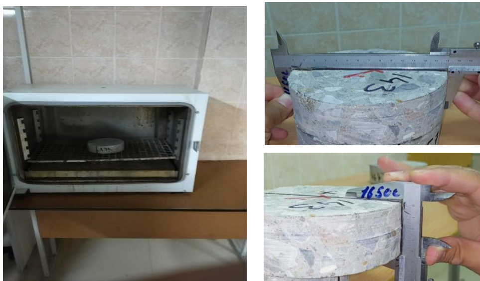
Figure 3. Thermal Testing of Concrete Samples
