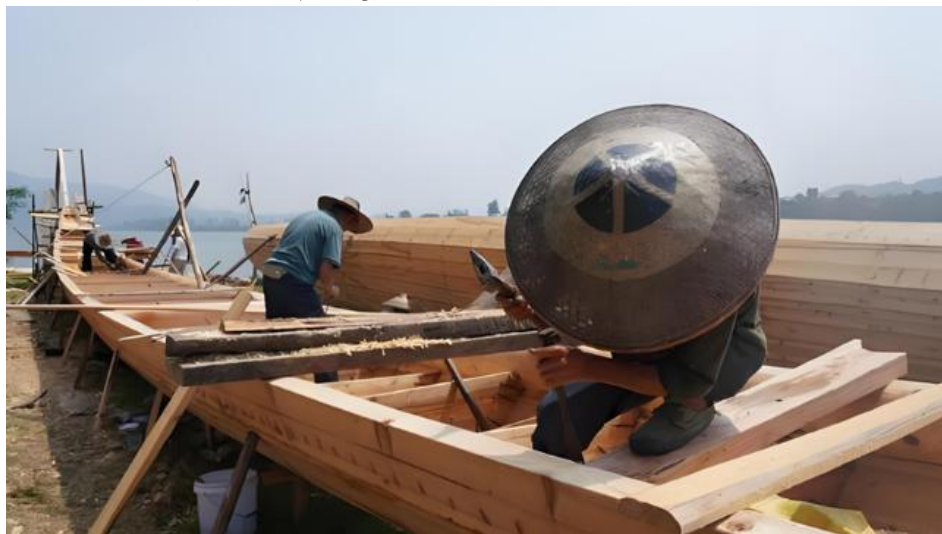
Fig. 12 The making of the cabin of the Miao people's wooden dragon boat.
