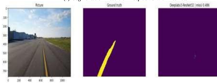
(b) Segmentation Result of DeeplabV3+ with ResNet32
