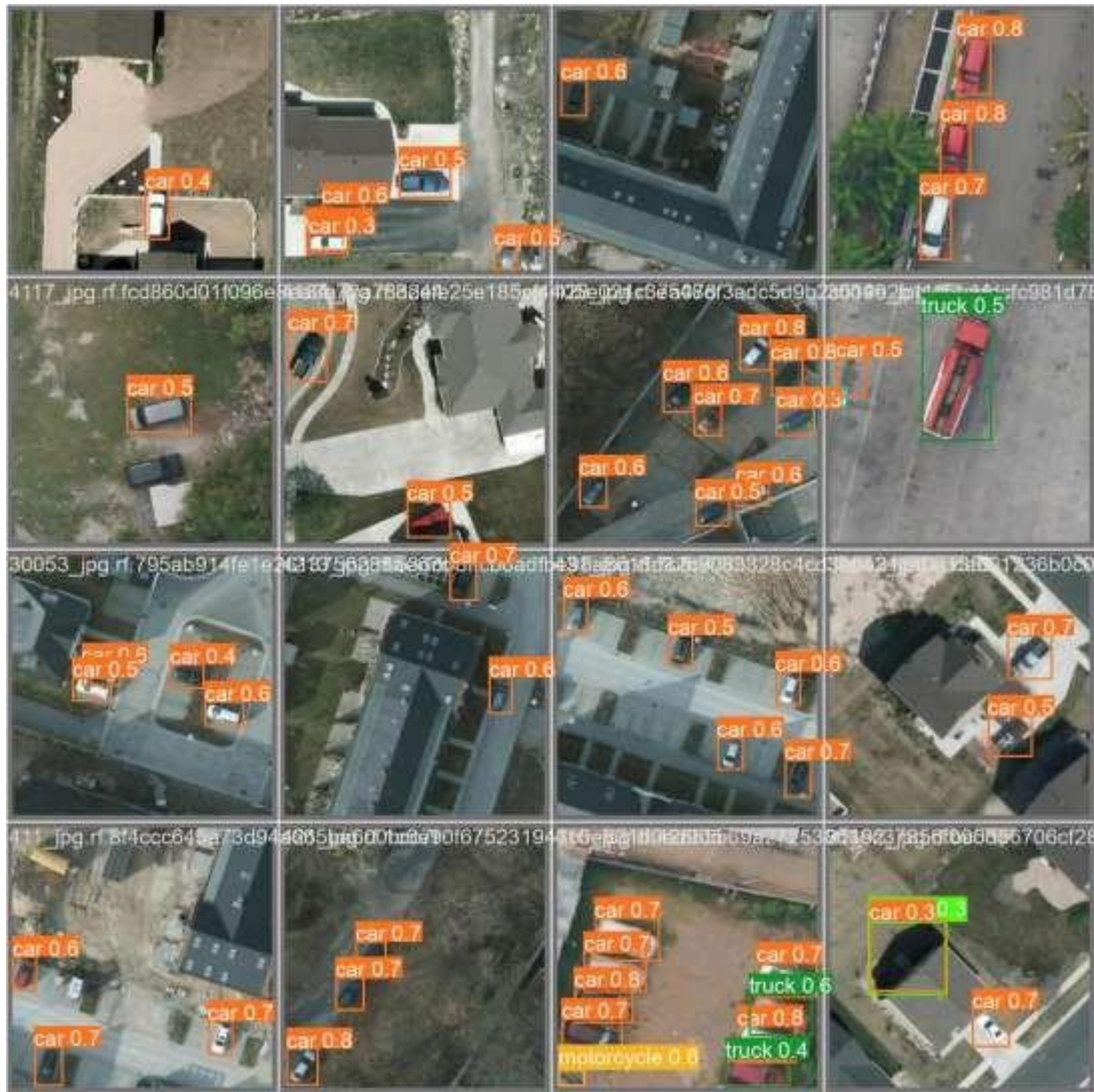
Figure 8: Proposed model Object Detection Results
