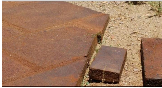
Fig.3 Ferrock slab and brick [10]
