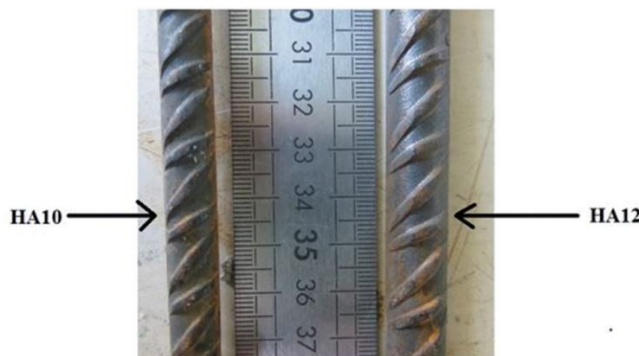
Fig.9 The bar specimens of steel rebars HA10 and HA12. [20]
