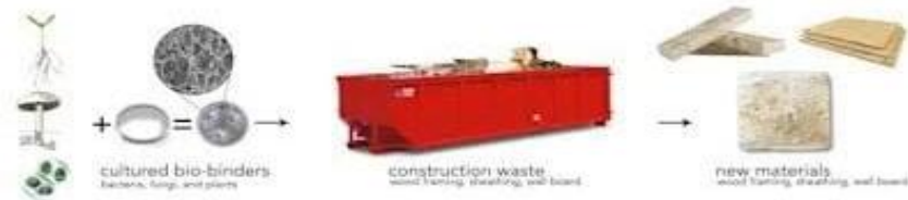
Fig.6 Bioterals diagram photo for new building material from Mycelium.
