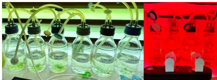
Figure 4. The medium in different pH and light supply for all the medium were put under the varied light with aeration continuously for 20 days.
