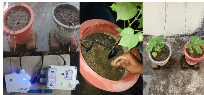
Fig. 1: Actual Experimental setup using cotton crop in black sandy loamy soil with sensors.
