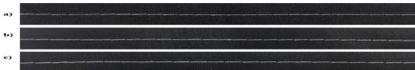
Figure 5. Image of seam appearance using Tex 24 thread, at stitch density of 3,5 stitches per centimeter using different needle sizes
