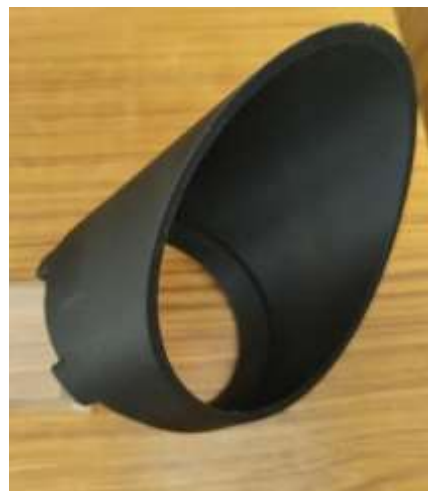
Fig.3. 3D printed model of Air intake connector
