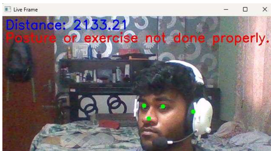
Fig. 4. Real-time feedback output, indicating incorrect posture with a red warning message, "Exercise Not Done Properly."
