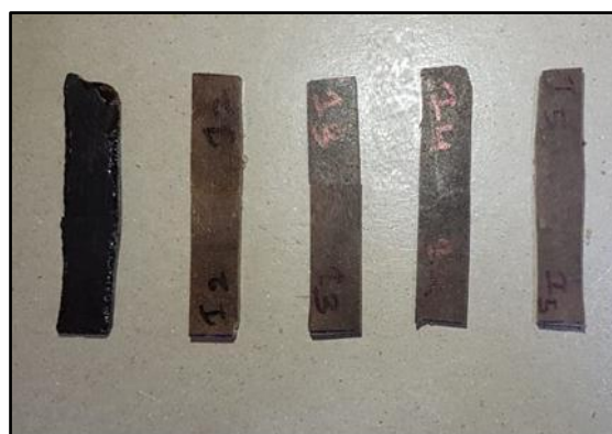
Figure4: Hybrid samples prepared according to ASTM D256 standard (Impact testing)
