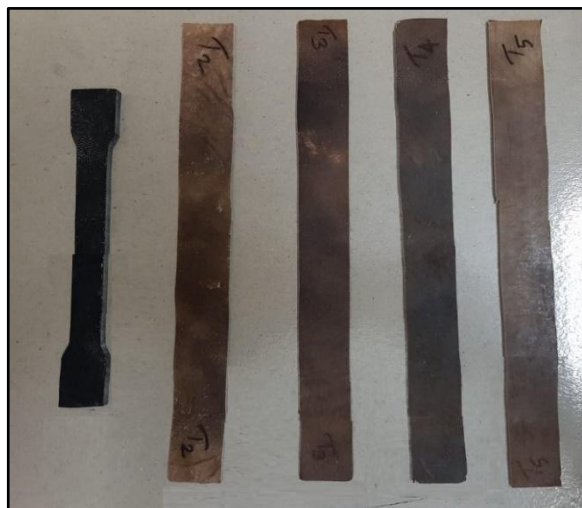
Figure2: Hybrid samples prepared according to ASTM D3039 standard (Tensile testing)
