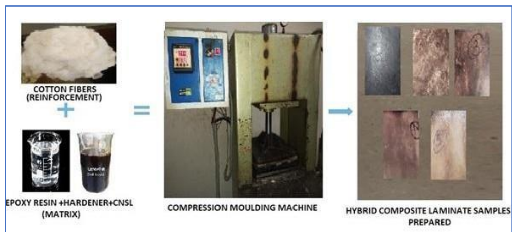
Figure 1. Laminated composite process
