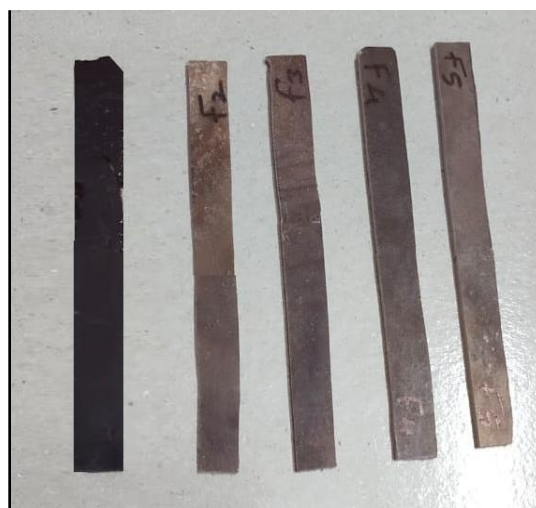
Figure3: Hybrid samples prepared according to ASTM D7264 standard (Flexural testing)
