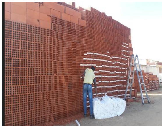
Figure 9: Insulated Clay Blocks for Construction
