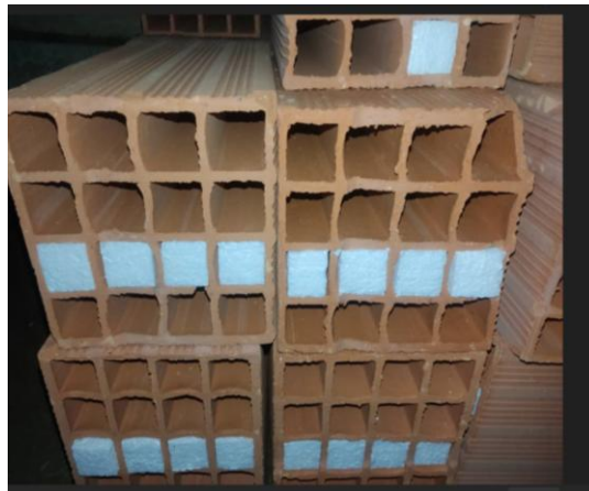
Figure 8: Insulated Clay Hollow Blocks with Polystyrene
