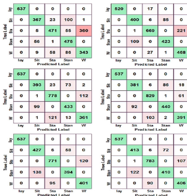
Fig. 8. Impact of UCI Data Point Removal on Activity-Specific Detection Accuracy for Linear Interpolation (left) and Cubic Interpolation (right) with Removal of One in Between (top), Two in Between (middle), and Three in Between (bottom).
