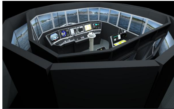
Figure 2. Full Mission Ship Handling Simulator – from above
