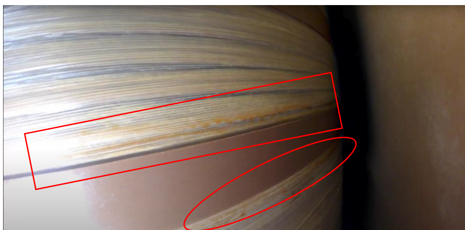
Figure 15. Spot Marks on the insulation paper of the HV Phase T Winding
