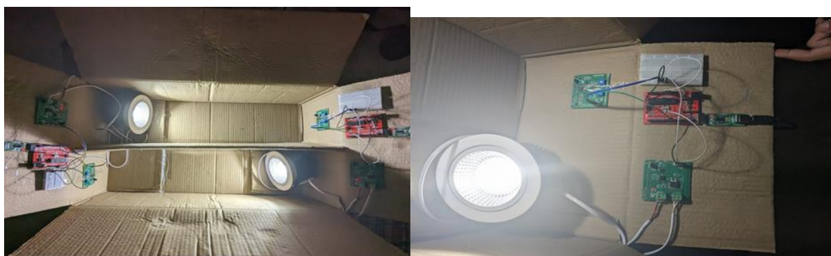
Fig. 4. Setup of LiFi communication (Prototype)
